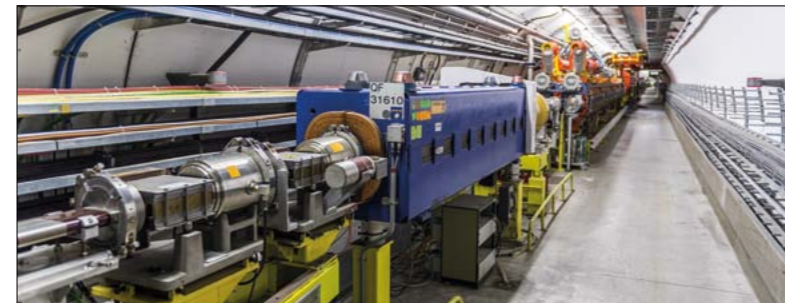
The SPS tunnel, with a quadrupole magnet in the foreground. (Image credit: CERN-GE-1311288-03.)
