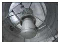
The cryostat for the XENONIT experiment. (Image credit: The XENONIT Collaboration.)
