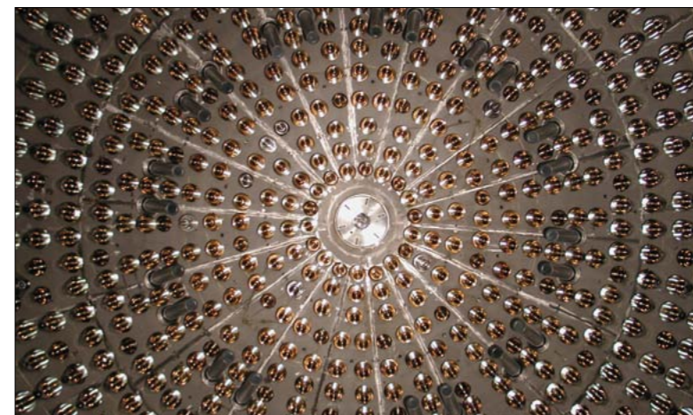
A total of 2212 8-inch photomultipliers mounted on a 13.7-m diameter stainless-steel sphere detect the scintillator light produced in Borexino. (Image credit: Borexino Collaboration.)
